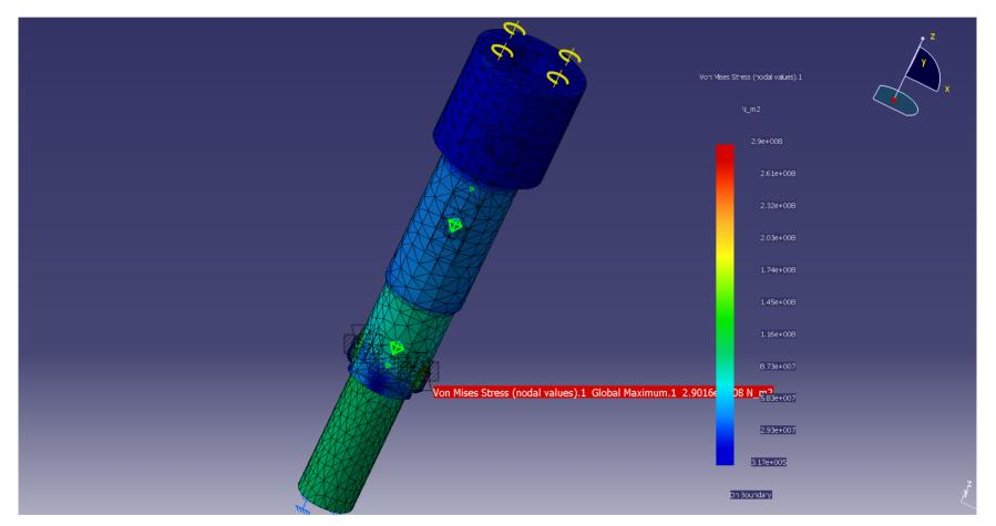
Stresses increase as one moves from the tool driver to the cross-pin and finally to the motor shaft. Smooth transition of the stresses takes place.
