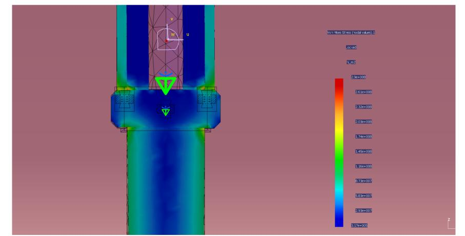
Detail view shows that max stresses are at the junction of motor shaft/tool driver/crosspin. However, the stresses are well below the yield strength of the material.
