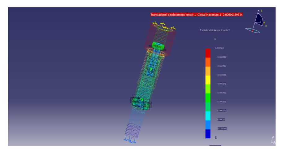
Displacement is maximum at the application point and least at the motor fixed end as one would predict
